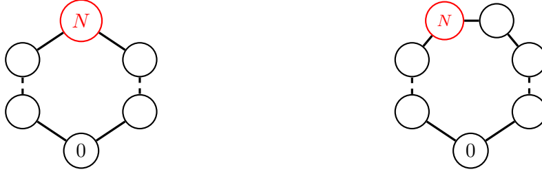
Figure 2: Quantum walk on a 2N -cycle (left), and on a (2N + 1) -cycle (right). We start from the state |0\rangle (with coin register on |\uparrow\rangle , and we want to reach the state |N\rangle ).
