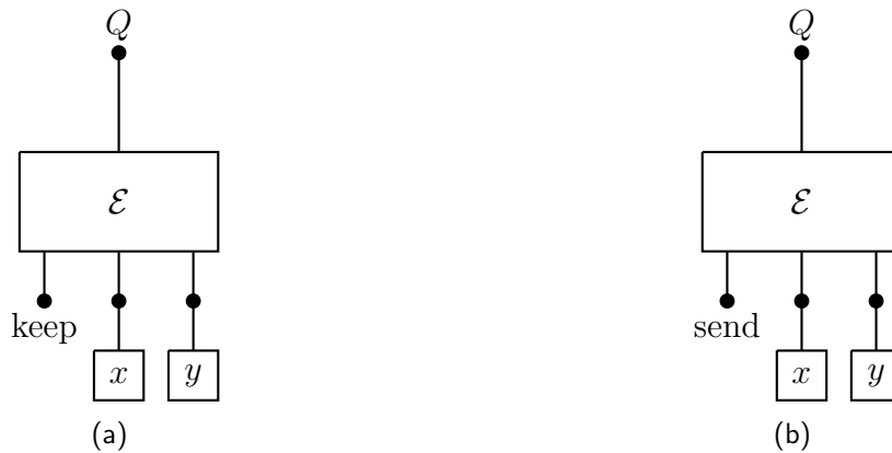
Figure 9: Some simple code-routing protocols. The map \mathcal{E} takes in the Q system and records it into a 3 share secret sharing scheme where any 2 shares recover the secret. The lower boxes indicate the share should be brought to the side labelled by the corresponding bit value, which we can achieve using a garden-hose protocol that uses O(1) EPR pairs. a) Code-routing protocol for computing AND(x, y) . b) Code-routing protocol for OR(x, y) . Figure reproduced from [23].
