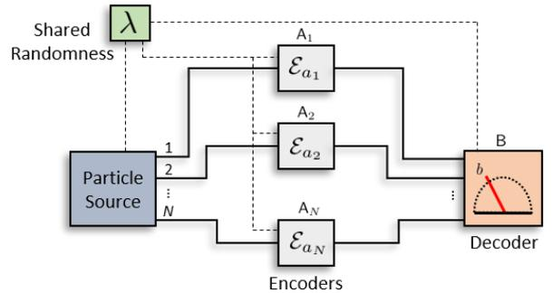
Figure 4: When randomness is shared between the source, the encoders, and the decoder, the generated channels have the form of Eq. (17). These MACs constitute the convex hull of  $\mathcal{C}_N$  and is denoted by  $\text{conv}[\mathcal{C}_N(\mathcal{A}, \mathcal{B})]$ .
