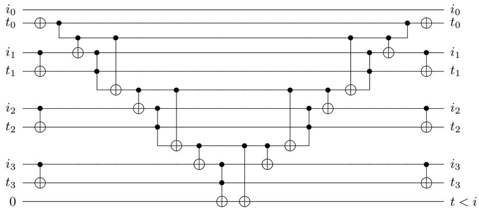
Figure 17: A circuit to perform an inequality test on 4 bits, with  $i$  given classically and  $i_0$  equal to 1. We can save one Toffoli, and the first ancilla is not needed because we can control directly on  $t_0$ .
