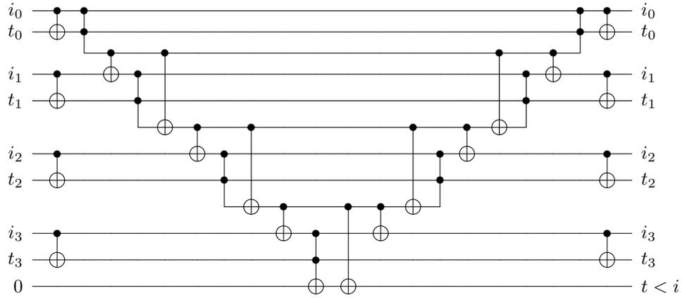
Figure 16: A circuit to perform an inequality test on 4 bits. This time the circuit restores the original values in the  $t$  registers, so it does not alter this register and just outputs the result of the inequality test.
