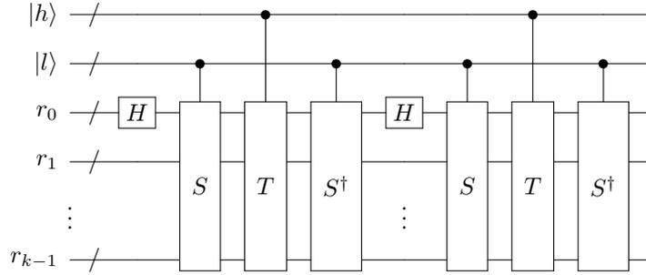
Figure 4: The sequence of operations used for computing table lookups with dirty ancillae. The output register is  $r_0$ , and the registers  $r_1$  to  $r_{k-1}$  are the dirty ancillae. Note that the scheme in [44] (see Fig. 1(d)) uses “SWAP” for the operation we here call  $S$ , and “SELECT” for the operation we here call  $T$ . The sequence of operations we use here is different than in [44], resulting in a reduction in the number of registers needed.
