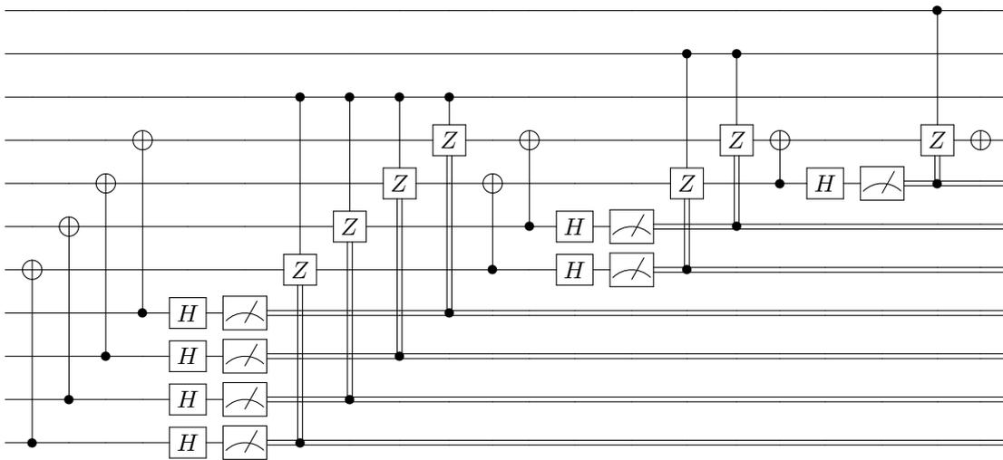
Figure 10: The circuit in Figure 9 with the Toffolis replaced with measurements and controlled operations, and the second CNOT in each group omitted.
