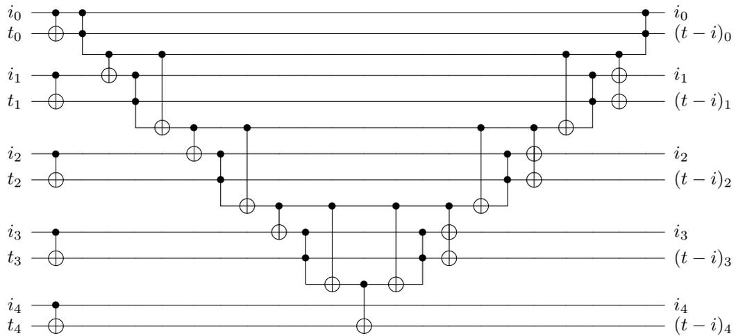
Figure 14: A circuit to perform subtraction on 5 qubits modulo  $2^5$ .
