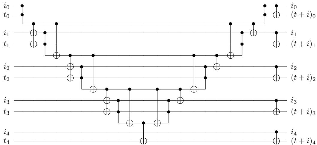
Figure 12: A circuit to perform addition on 5 qubits modulo  $2^5$ . This circuit is also sufficient for non-modular addition if we know there will not be overflow.
