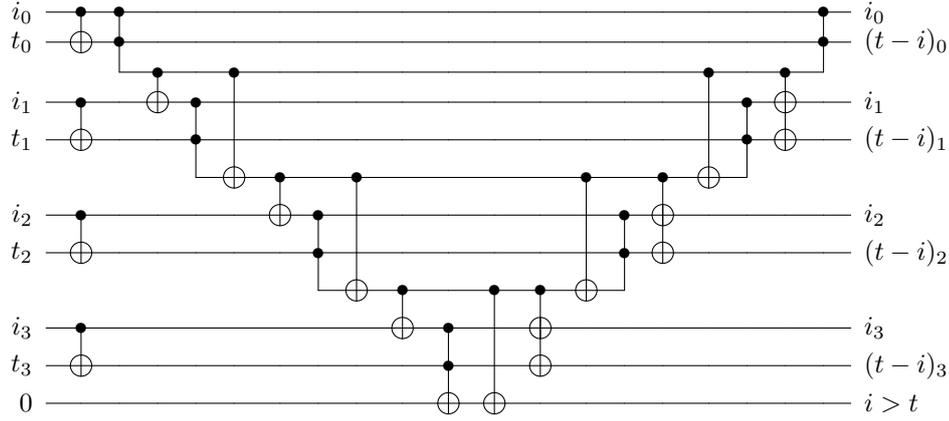
Figure 15: A circuit to perform an inequality test on 4 qubits. The output bit is  $(t - i)_4$ , and will be 1 if  $t < i$ . This is because it performs modular subtraction on 5 bits, with  $i_4$  and  $t_4$  guaranteed to be zero. The maximum values of  $i$  and  $t$  are 15. If we subtract  $i$  from  $t$  modulo 32, and  $t < i$ , then the result will be between 17 and 31. These numbers all have bit 5 equal to 1.
