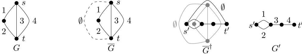
Figure 1: Example of how to derive \bar{G} , \bar{G}^\dagger , and G' from a planar graph G where s and t are on the same face. \bar{G} is obtained from G by adding an edge (\{s, t\}, \emptyset) . \bar{G}^\dagger is the planar dual of \bar{G} . (In the diagram labeled by \bar{G}^\dagger , \bar{G} is the gray graph, while \bar{G}^\dagger is black). G' is obtained from \bar{G}^\dagger by removing the edge (\{s, t\}, \emptyset)^\dagger . Note that dual edges inherit their labels (in this case 1, 2, 3, 4, \emptyset ).
