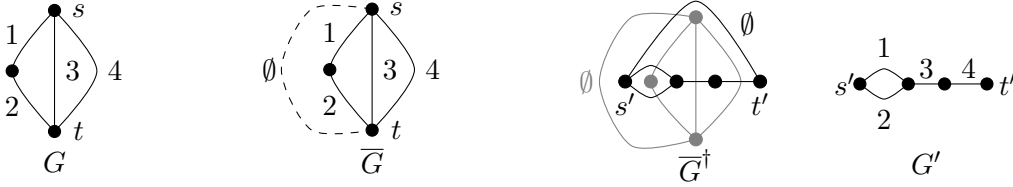
Figure 1: Example of how to derive \overline{G} , \overline{G}^\dagger , and G' from a planar graph G where s and t are on the same face. \overline{G} is obtained from G by adding an edge (\{s, t\}, \emptyset) . \overline{G}^\dagger is the planar dual of \overline{G} . (In the diagram labeled by \overline{G}^\dagger , \overline{G} is the gray graph, while \overline{G}^\dagger is black). G' is obtained from \overline{G}^\dagger by removing the edge (\{s, t\}, \emptyset)^\dagger . Note that dual edges inherit their labels (in this case 1, 2, 3, 4, \emptyset ) from the primal edge.
